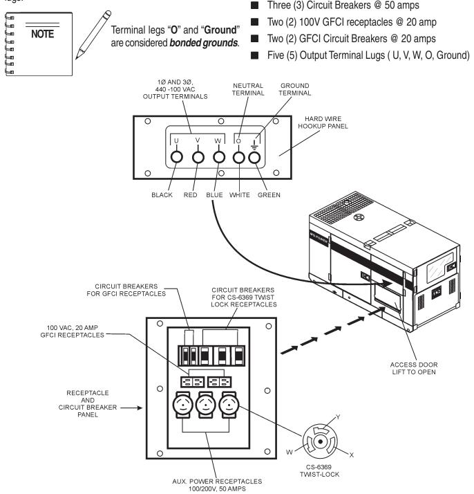
Figure 8. Output Terminal Panel
